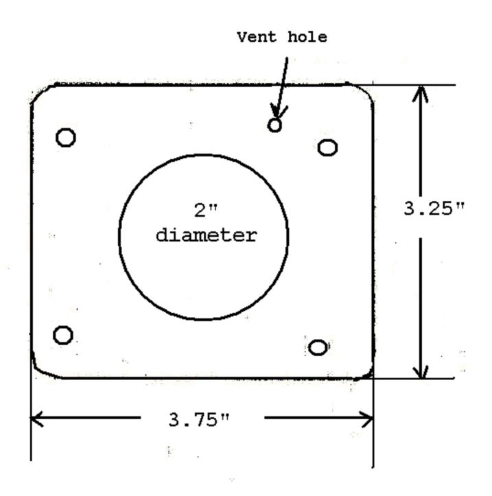
This plate replaces the existing backing plate. You must remove the collar and bearing from the axle to install
