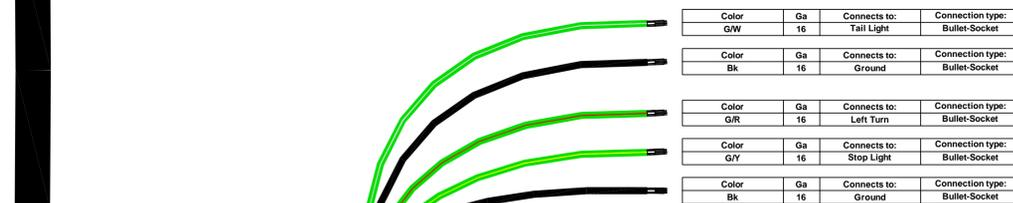
Note: The ground wire is two 16 gauge wires that branch to all the ground wires.
