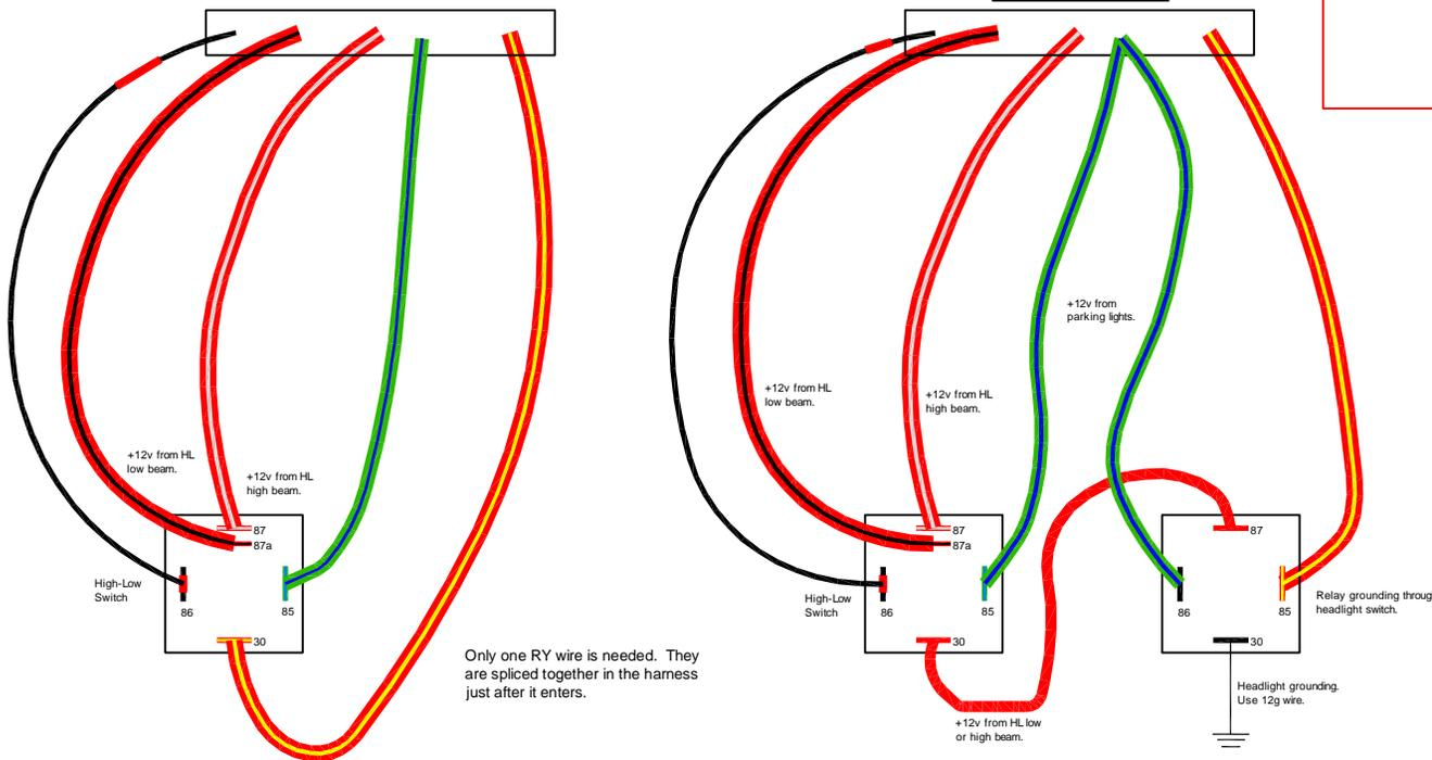
Only one RY wire is needed. They are spliced together in the harness just after it enters.
