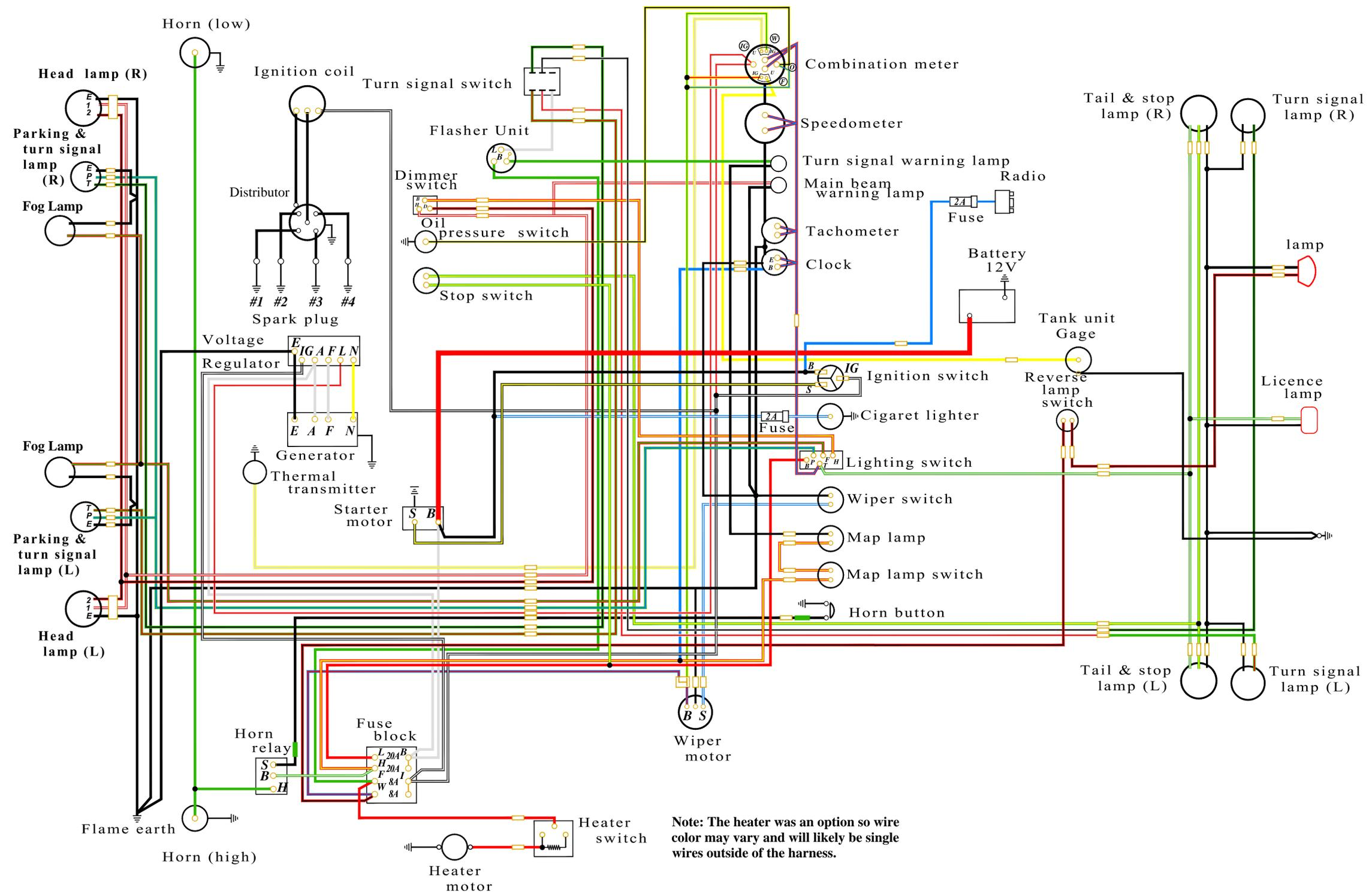
**Note: The heater was an option so wire color may vary and will likely be single wires outside of the harness.**
