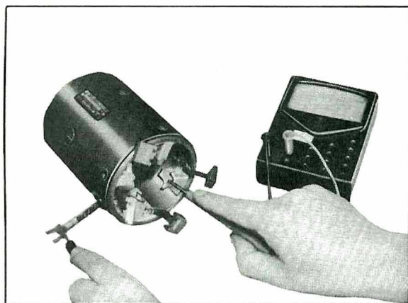
Fig. EE-58 Field Coil Test for Continuity
