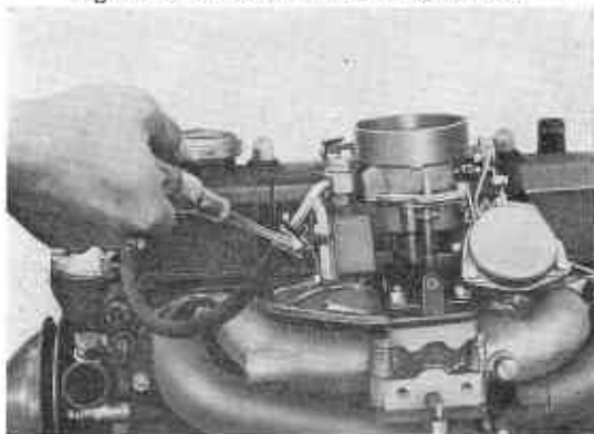
Fig. EF-3 Removing Piping
