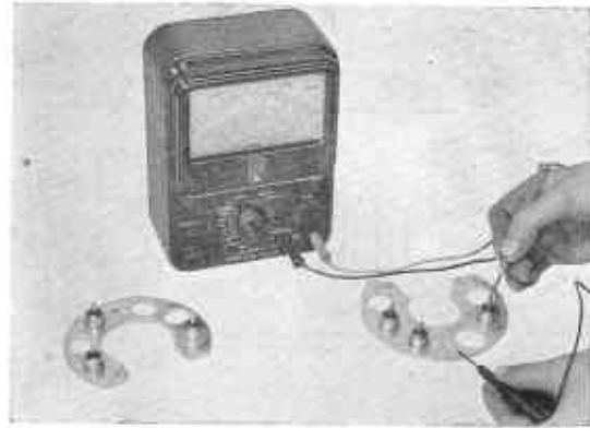
Fig. EE-27 Inspecting Individual Diode
