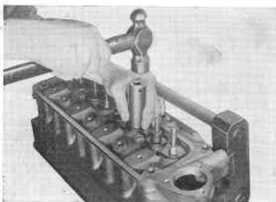
Fig. EM-42 Installing Lip Seals
