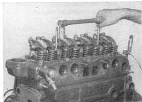
Fig. EM-4 Removing Rocker Shaft Assembly
