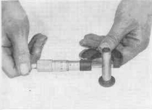
Fig. EM-38 Measuring Valve Lifter Diameter
