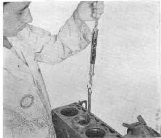
Fig. EM-26 Checking Piston-to-Cylinder Wall Clearance
