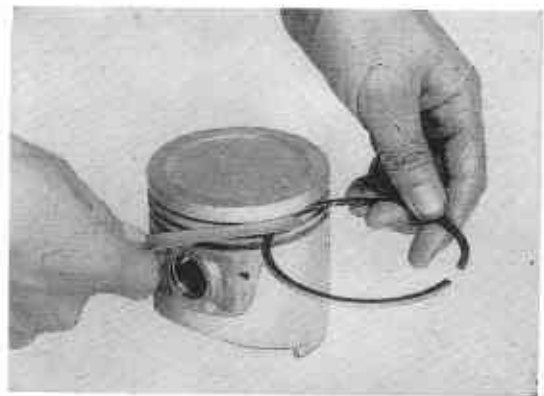
Fig. EM-27 Checking Piston Ring-to-Groove Land Clearance
