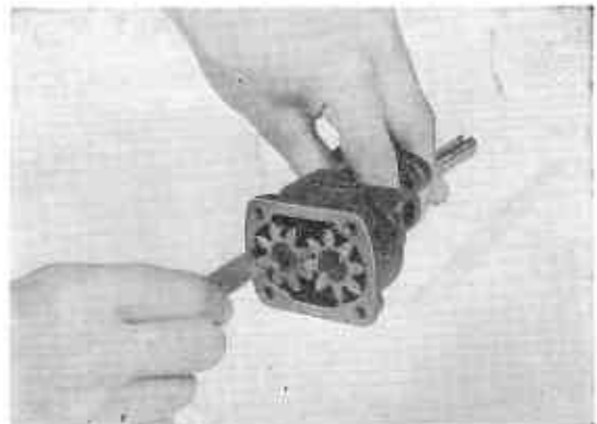
Fig. EL-4 Checking Clearance between Body and Gear
