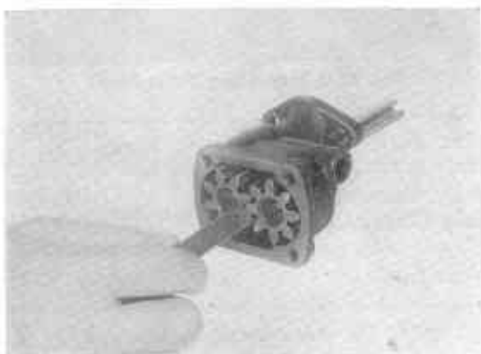
Fig. EL-5 Checking Gear Backlash
