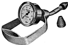
Fig. 1 Measuring Compression Pressure by Means of a Compression Gauge
