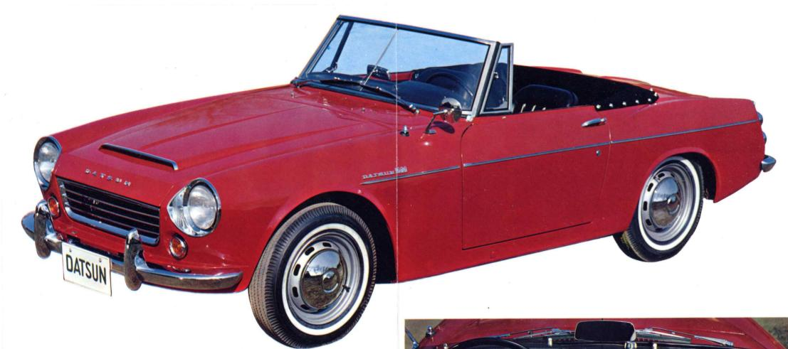
1,600 cc (97.3 cu. in), 96 HP engine 4-speed full-synchromeshed transmission Max. speed 106 MPH Front wheel disc brakes
