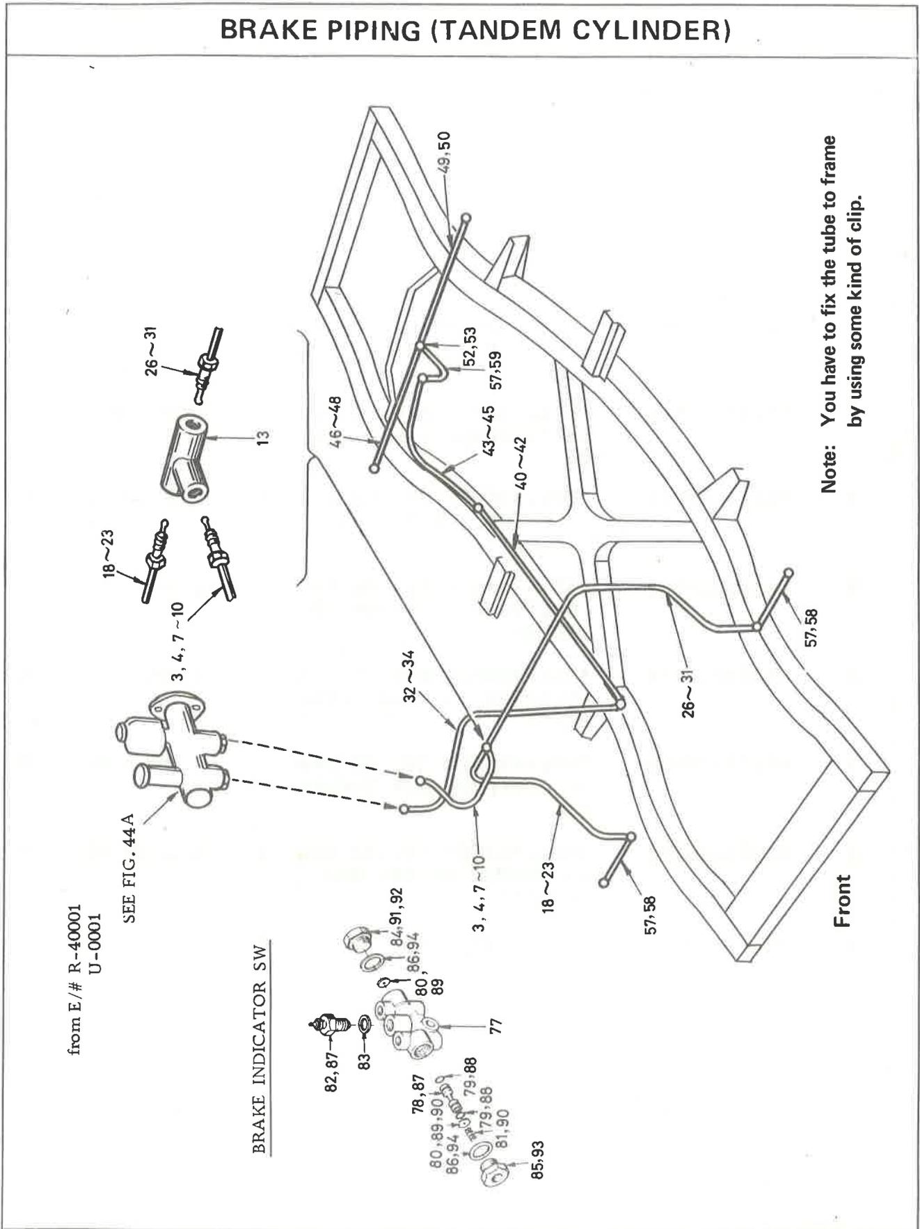
Note: You have to fix the tube to frame by using some kind of clip.
